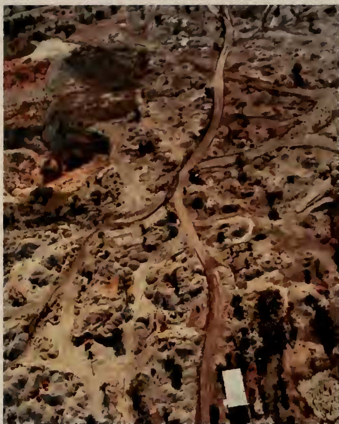
Figure 4. Aerial shot taken in 1994 showing opal workings in the Preserved Opal Fields. Underground mining is evidenced by mullock heaps stored on the ground surface, and part of the historic Western Fall open cut mine can be seen at the top of the photograph. (Photographer: Dave Barnes; Industry & Investment NSW photographic library).
